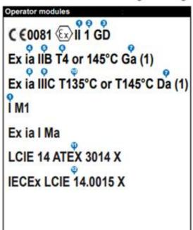
+ cable link 9 9 9 € € 0081 (Ex) II 1 GD Ex ia IIB T4 or 145°C Ga (1) Ex ia IIIC T135°C or T145°C Da (1) IM1 Ex ia I Ma Ui: 5.9V; Ii: 210mA; Pi: 310mW; Ci: 96.2µF; Li: 0.54µH **LCIE 14 ATEX 3014 X** IECEX LCIE 14.0015 X
